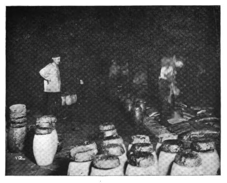
Hot work. Placing full crucibles in furnaces
